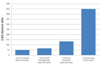
In accordance with the ASTM E-1300 protocol (calculated 0.8% probability of failure), Corning Gorilla Glass demonstrated superior bending strength, enabling the use of thinner glass to support the same load when compared to soda-lime glass.
