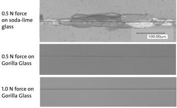
When subjected to a scratch resistance test involving loads of 50g of force (Knoop indenter), Corning Gorilla Glass showed greater scratch resistance compared to air tempered soda-lime glass. All results shown at same magnification.
