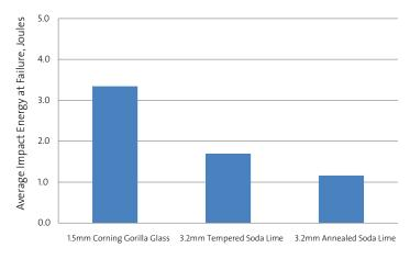
Data is based on ball-drop impact with 535g steel ball.
